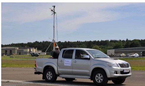
Figure 3: Channel sounder mounted on car
